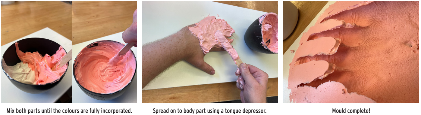
Mix both parts until the colours are fully incorporated.
