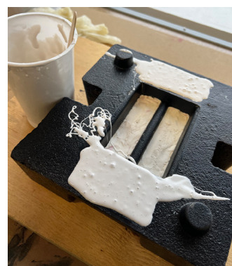
Great for casting with deep undercuts like the underside of a Stage Weight.
